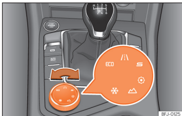
Sl. 173 Sredinska konzola: vrtljivi gumb Driving Experience.
